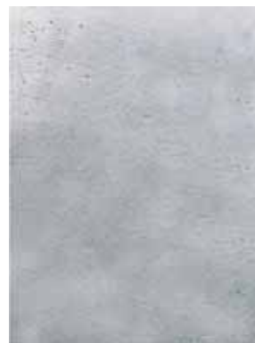
Sikaflex® AT Façade after 2000 hours QUV
